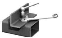
Using an open-end wrench on the outside of the steel plate to tighten the washerand apply torque to the hexagon head by a torque wrench.
