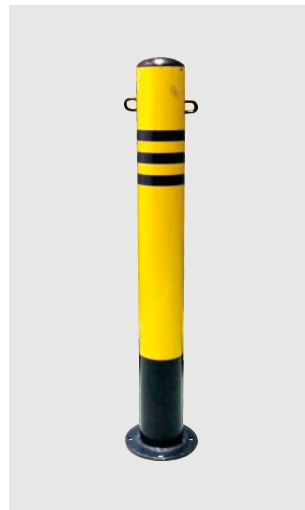
Name: Protective Pile (Fixed) Model: TLJT-FHZ01-EH Specification: \phi 76 \times 600 \text{mm} \phi 89 \times 750 \text{mm} , \phi 114 \times 1000 \text{mm} Material: high quality steel pipe, high pressure spraying Engineering grade reflective film Application: road entrance
