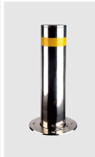
Name: Protective Pile (Fixed) Model: TLJT-FHZ04 Specification: \phi 133 \times 600 \text{mm} Material: high quality steel pipe, high pressure spraying Engineering grade reflective film Application: road entrance
