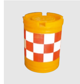
Name: Anti-collision bucket Specification: \phi 600 \times 800 \text{mm} Material: FRP Model: TLFZT-02 Application: road bifurcation
