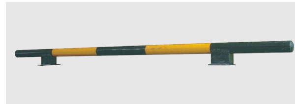
Name:Welded parking wheel Model:TLJT-DLGOI Specifications:φ60X2000mm/φ76X2000mm/φ89X2000mm Material:mirror zinc steel pipe, high pressure spray coating, engineering grade reflective film Application:parking spaces
