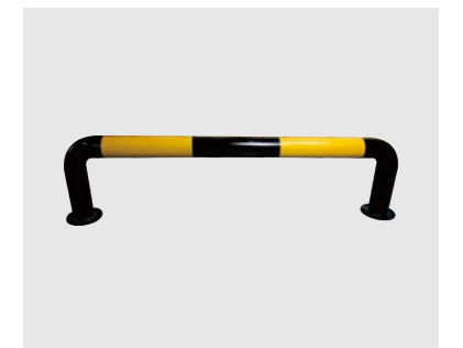
Name: U-shaped guardrail Model: TLJT-UHL01 Material: high quality steel pipe, high pressure spraying Engineering grade reflective film Specification: \phi 38 \times 1500 \times 1050 \text{mm} Application: aisle
