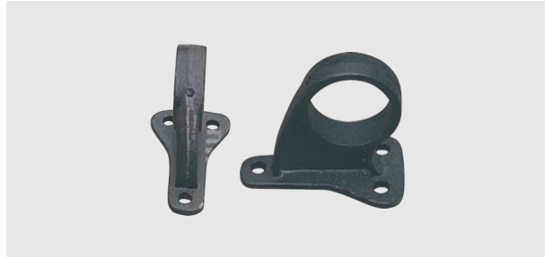
Name:Perforation in the middle of the parking wheel block (three screw holes) Model:TLJT-3TJ01-ZJ Specifications:φ60/φ76/φ89 Material:cast iron Application:parking spaces
