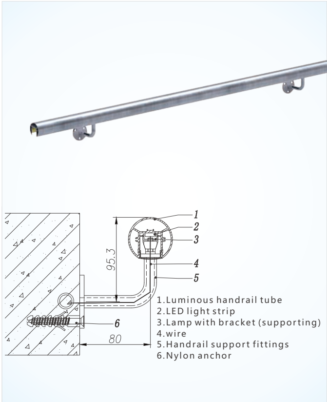
HSG01-G Luminous handrail tube Material: 6063-T6 L≤5700mm
