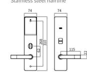
Main material: stainless steel Applicable door thickness: 40-50mm, customized when exceed.
